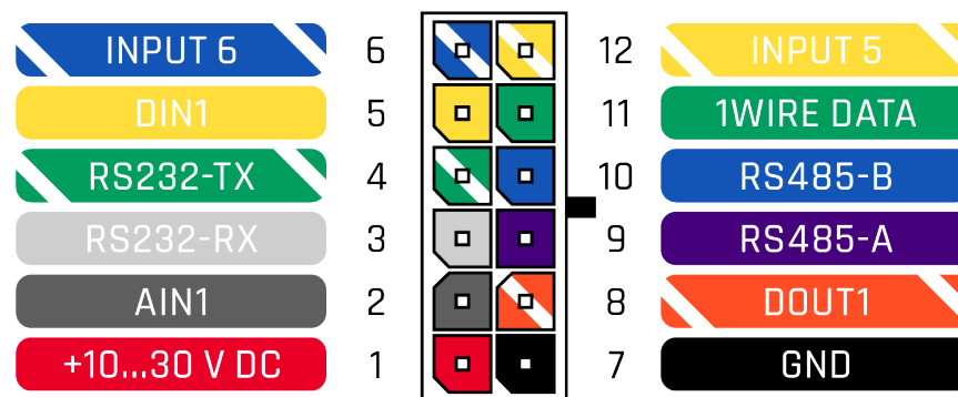
Figure 2 FMB125 2x6 socket pinout
