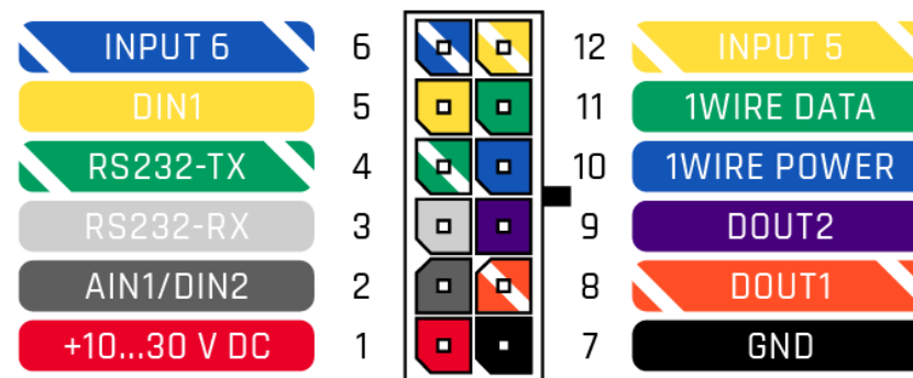
Figure 2 FMC125 2x6 socket pinout
