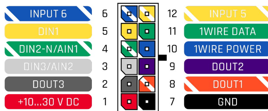
Figure 2 FMC130 2x6 socket pinout
