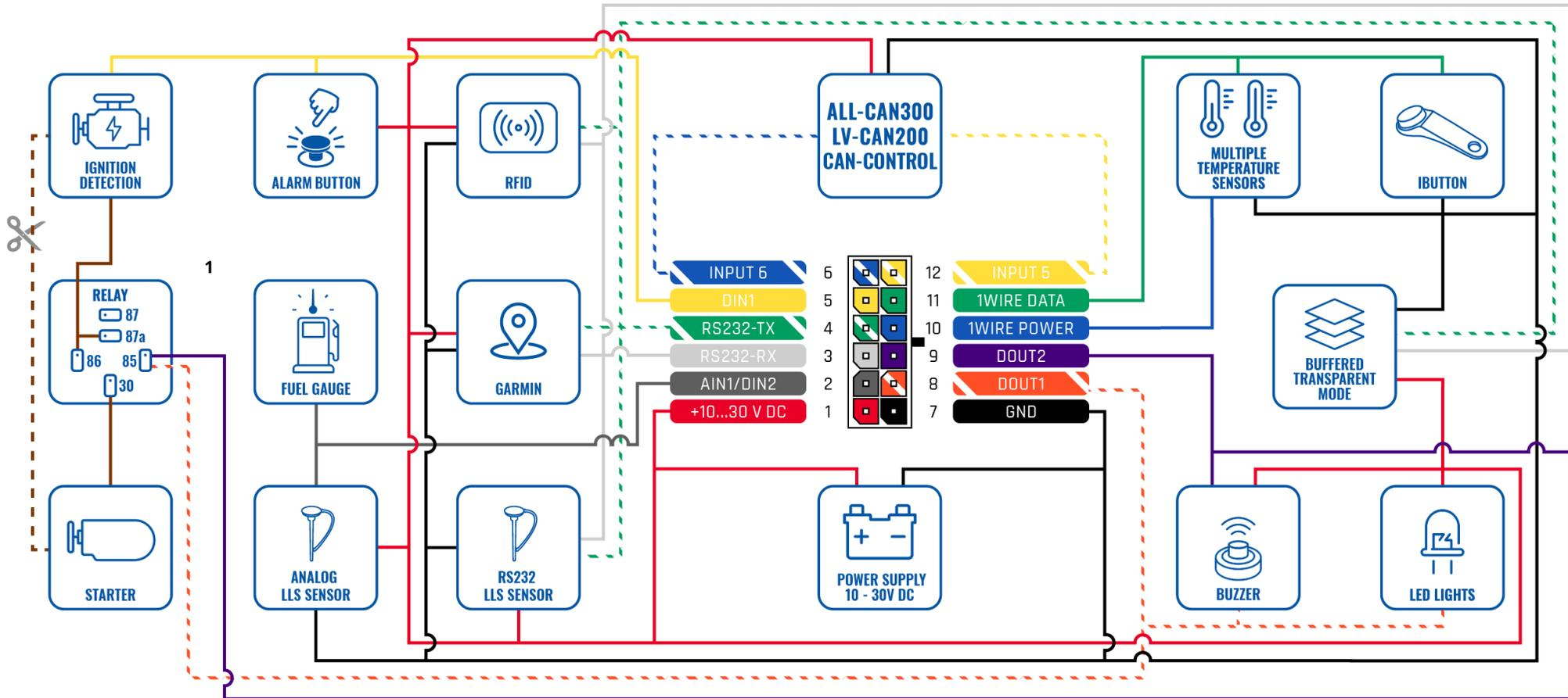
Figure 3 FMM125 Wiring scheme
