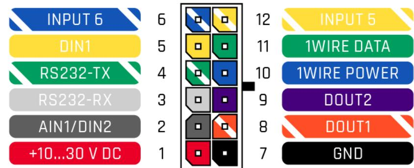
**Figure 2 FMM125 2x6 socket pinout**
